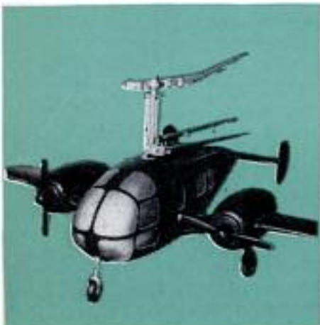
Coaxial rotors of the Navy model fold for storage on carrier
